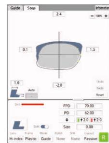
To further enhance precision, the ME-1 features variable step angle control, which maintains a uniform step width across the entire lens shape. This prevents the base of the step from becoming thinner, which leads to a consistent accurate fit, even in complex frame geometries, delivering professional-grade results with every lens.
